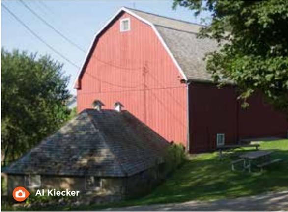
The **barn** was built in 1928, replacing one that was destroyed by fire. The concrete foundation walls were made with rocks and sand from the farm mixed with cement. The post and beam construction of the barn makes for a very strong building.
